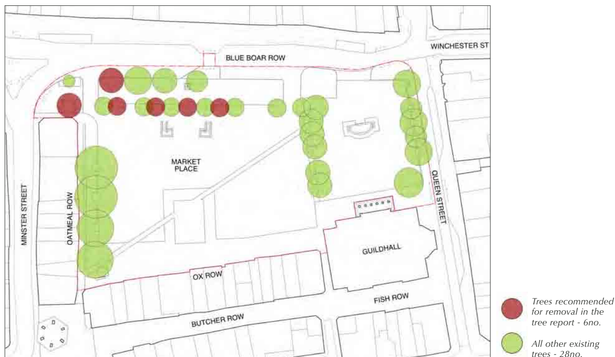
Plan highlighting the existing trees proposed for removal in the Duramen Tree Survey Report
